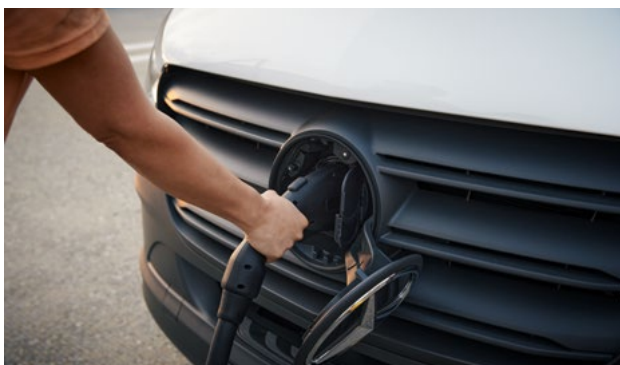
CCS rapid charging port, 115kW max. capacity.
