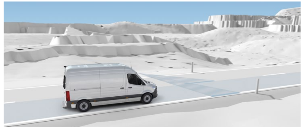
Illustration of Active Lane Keeping Assist.
