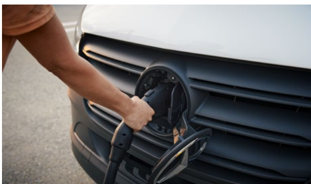
CCS rapid charging port, 115kW max. capacity.
