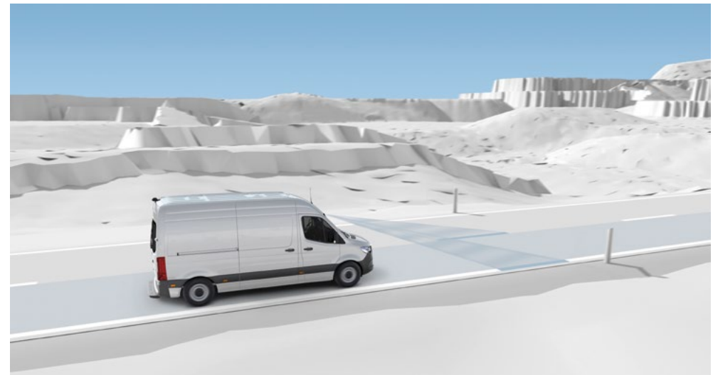
Illustration of Active Lane Keeping Assist.
