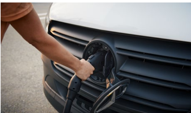
CCS rapid charging port, 115kW max. capacity.
